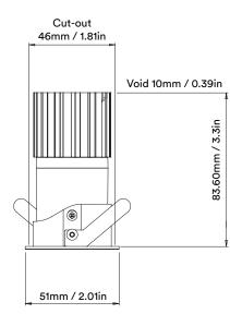
Unit height increases by 12mm / 0.48in for SPOT and both ELLIPTICAL BEAMS
